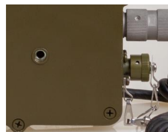
Side panel with MRJ (RJ45) connectors
