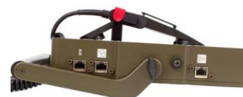
Side panel with MRJ (RJ45) connectors
